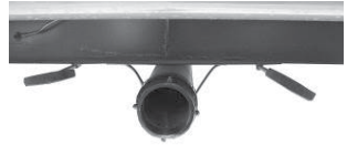
Black/Grey tank drain & valves
